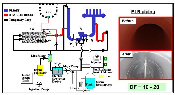
Fig. 3 Application of T-OZON to system decontamination in a BWR
