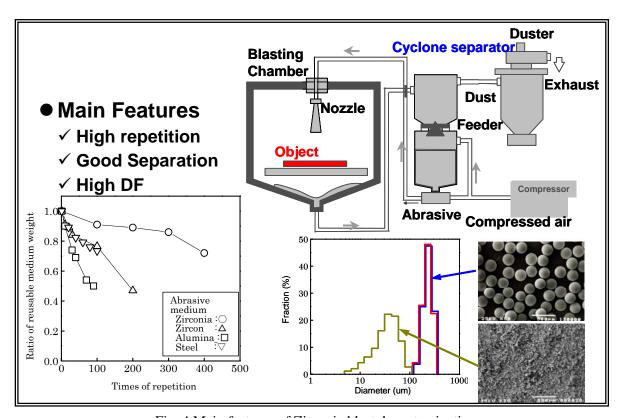
Fig. 4 Main features of Zirconia blast decontamination
