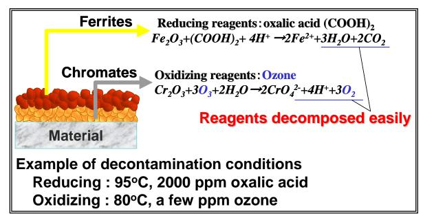
Fig. 2 Principle of T-OZON
