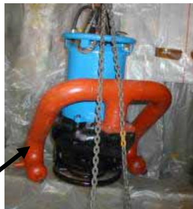
Discharge device in orange was attached to the pump
